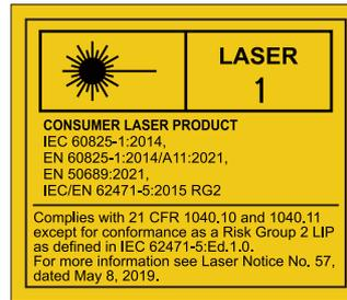
Above laser caution is located on the bottom of this apparatus.
