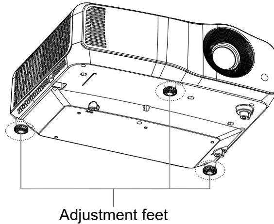
The projector is equipped with 3 adjustment feet to adjust the image height. To raise or lower the image, turn the adjustment feet to fine-tune the height.
